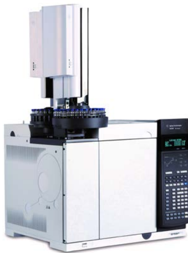
Figure 1 – Fully Automated Dual Channel 7890B GC Configured for UOP 411-13
