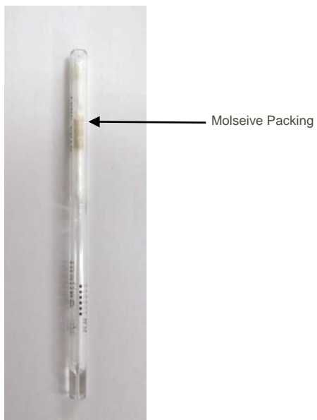
Figure 3 - Special Glass Inlet Liner with Molsieve Packing (Separation Systems, Inc. Part No. SS-053-500)
