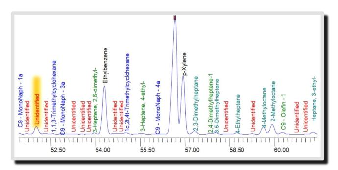
This diagram represents a small section of a DHA chromatogram showing identified components and 'undefined'. Hydrocarbon Expert™ dramatically simplifies the identification of undefined components using reference component database templates.
