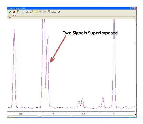
This capability is useful when differences between the reference signal and sample signal are not easily discerned. In this mode the superimposition of the signals can be adjusted by a single pixel to make sure they are clearly aligned.
