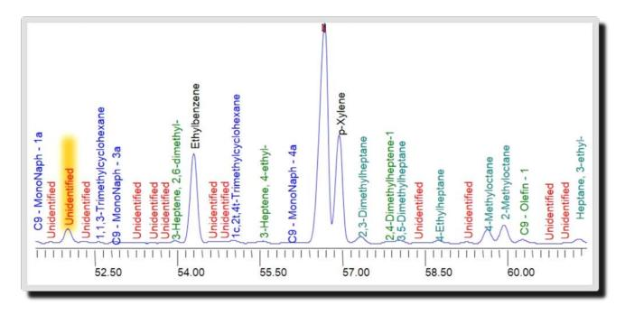
This diagram represents a small section of a DHA chromatogram showing both identified and 'undefined' components. Hydrocarbon Expert™ dramatically simplifies the identification of undefined components through the use of built in component name/retention time database templates. Templates that can be easily used to establish your own DHA database.
